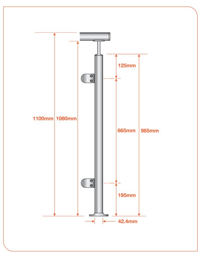
BALUSTRADE **Stainless Steel End Post** WITH SADDLE Code: PRSS316EPOST1060MM-42MM
