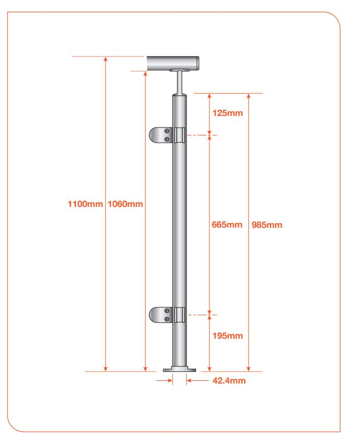
BALUSTRADE **Stainless Steel Corner Post** WITH SADDLE Code: PRSS316CPOST1060MM-42MM
